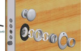
Check the thickness of the door and that the diameter of the hole is at least 50 mm otherwise drill the panel with a bevel cutter
